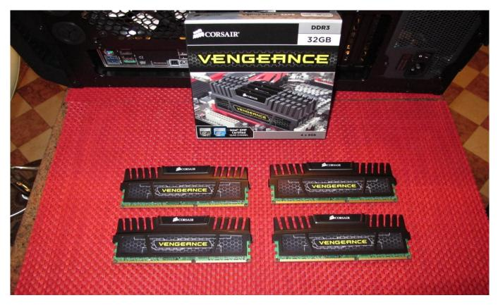
I then simply attached the first two ram units on the left side of the CPU - using pressure and a clam - below the cooling system. I then attached the second fan to the cooling system and affixed it with long screws. This is because the second fan is right above the RAM Units. I then clamped the remaining two Units to the rightr of the CPU.
