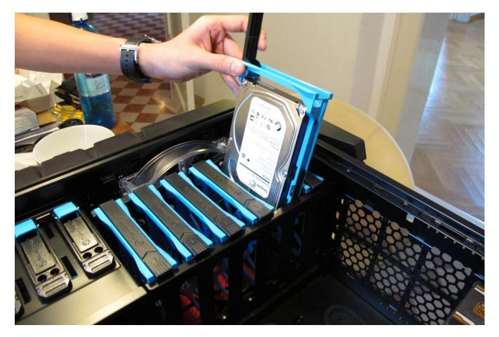
The Constellation hard drive wasn't the only hard drive that was used in the assembling. The PX-256M5P 2,5" SSD 256 GB Solid State Drive was also used in the building process. The black slot was needed because the SSD Drive was too small for the regular slot.
