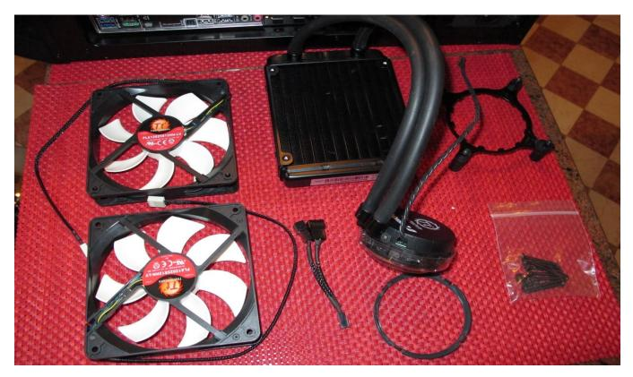
I detached the standard fan and replaced it with a Thermaltake fan for measurement reasons. I then placed the water cooling unit on top of the fan and attached it using screws. Notice that the second fan is not attached yet. I then affixed the liquid cooling capsule to the top of the CPU clamp using big screws and a ring for stabilization. The cooling liquid on top of the CPU was used as well.
