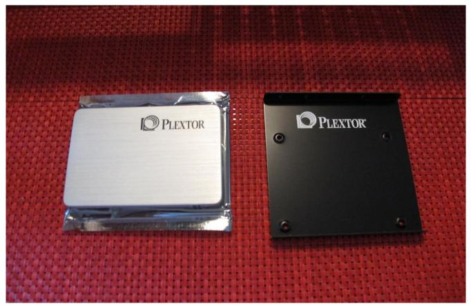
I placed the suited black Pextor slot into the original slot and affixed them using screws. Then the actual SSD Drive into the Plextor slot and attached it using built-in screws.
